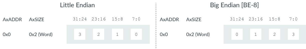
Figure 7-12: Little-endian and big-endian representations of the same four-byte word
