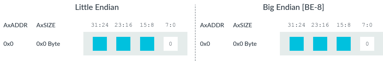
Figure 7-14: For a single byte, there is no difference between little-endian and big-endian mode
