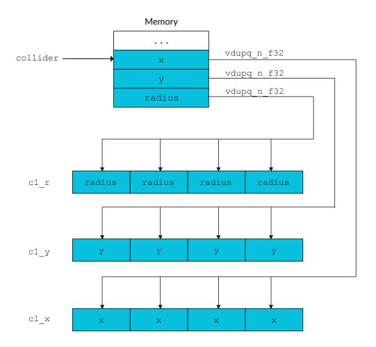
2. Load the x and y data for the next four input circles into separate lanes of two different Neon registers:
