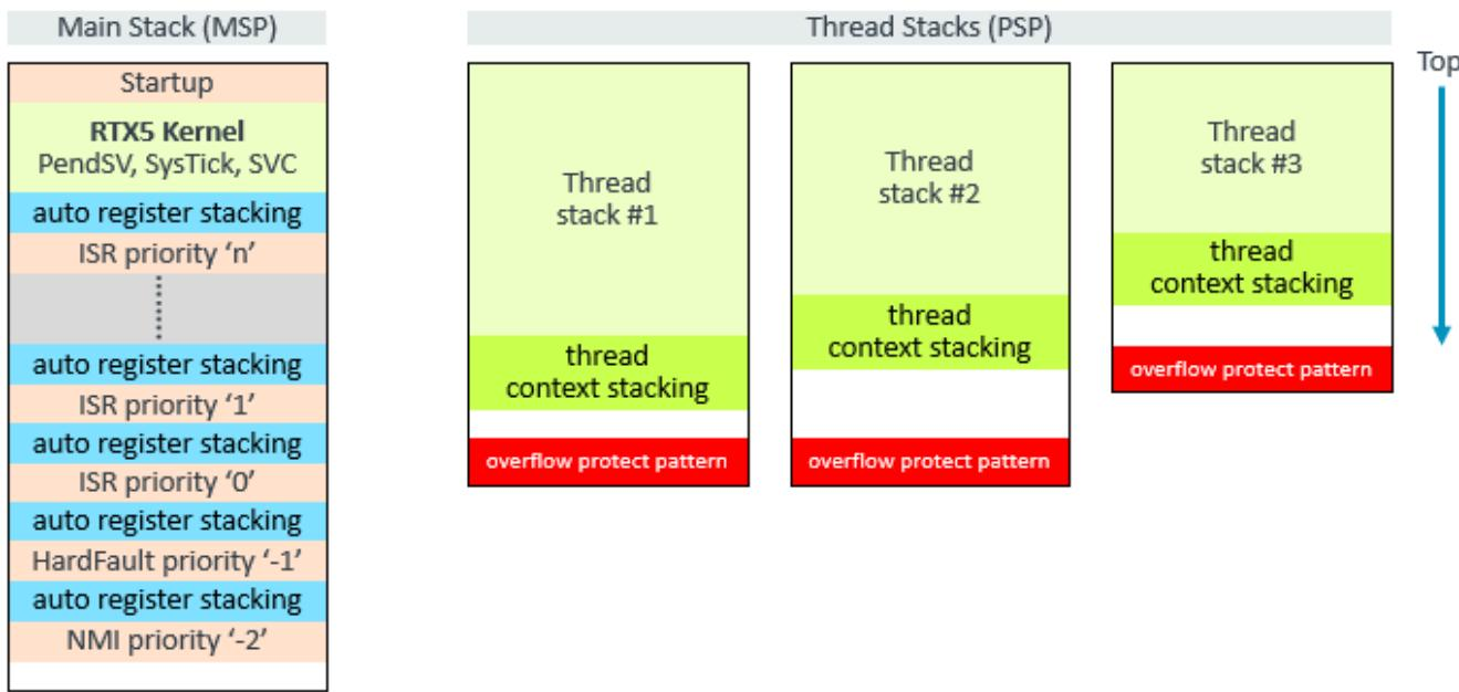
Note that RTX5 itself executes in handler mode and uses the *main stack* for kernel functions. This is different from other RTOS kernels (i.e. FreeRTOS), where the kernel functions use the *thread stack* and therefore require additional memory space on each individual *thread stack*.
