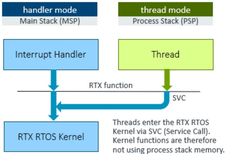
The RTX5 Kernel uses the following interrupt service routines:
