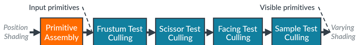
Figure 4-1: Arm 5 th Generation GPU culling pipeline
