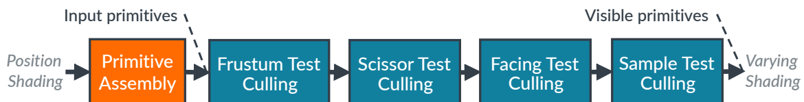
Figure 4-1: Arm 5 th Generation GPU culling pipeline
