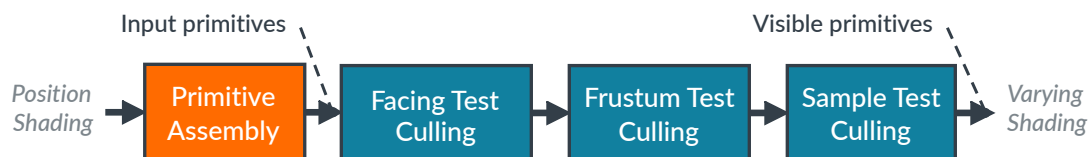
Figure 4-1: Valhall GPU culling pipeline
