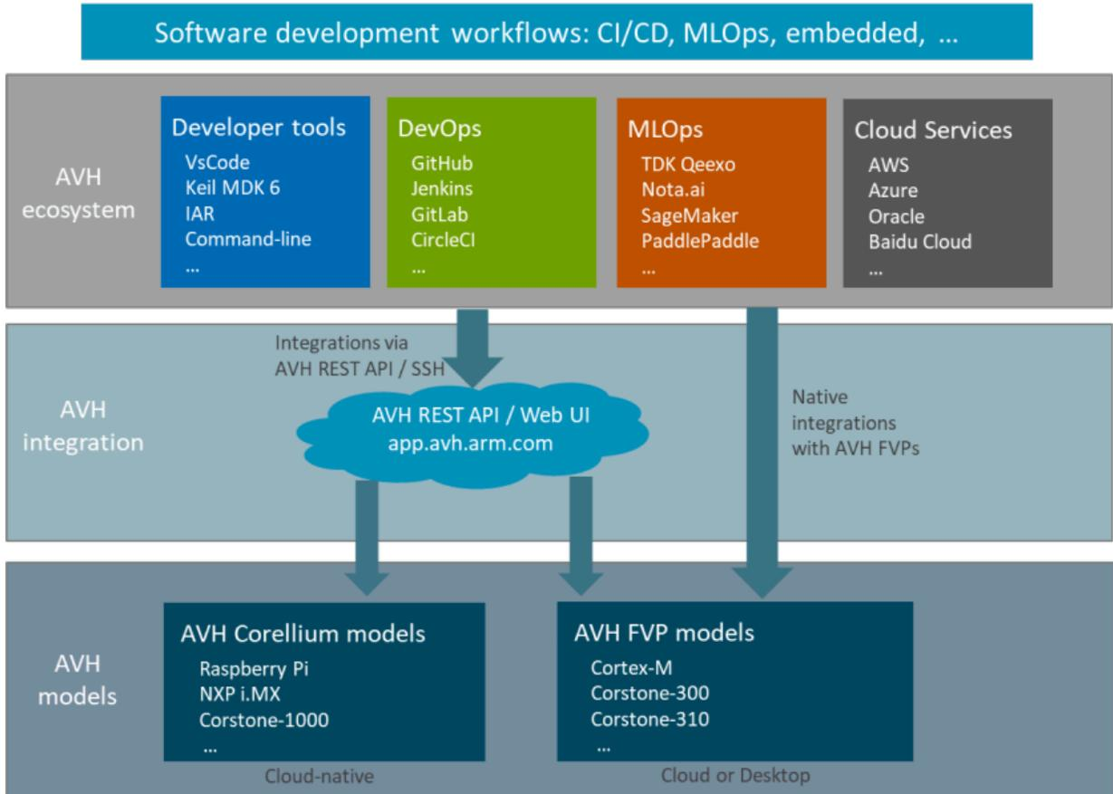
You can start developing and testing your applications on AVH ahead of silicon availability, and without having to spend time and money setting up and maintaining physical board farms. AVH provides an accurate simulation of Arm-based SoCs, enabling seamless transfer from a virtual model to your target hardware.
