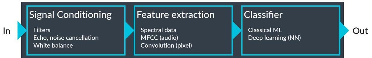
CMSIS-Stream provides tools to create optimized DSP pipelines, which are required to optimize ML software stacks. The visual representation that a compute graph provides can be helpful in complex DSP or ML workflows with multiple interconnected components, such as the one shown in the following diagram.
