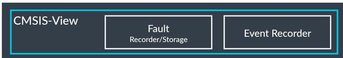
CMSIS-View helps you to see how your embedded systems are operating, with minimal memory and timing overhead. The event statistics functions enable you to collect and analyze statistical data about the execution of your code.
