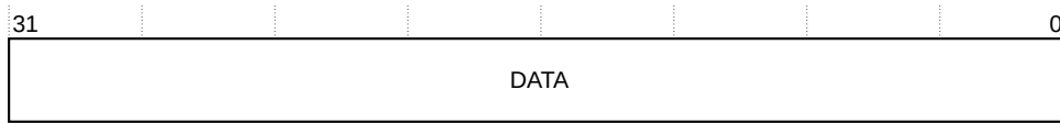
Figure 5-14: DCAICRR and DCADCRR bit assignments when reading the instruction or data cache data RAM
