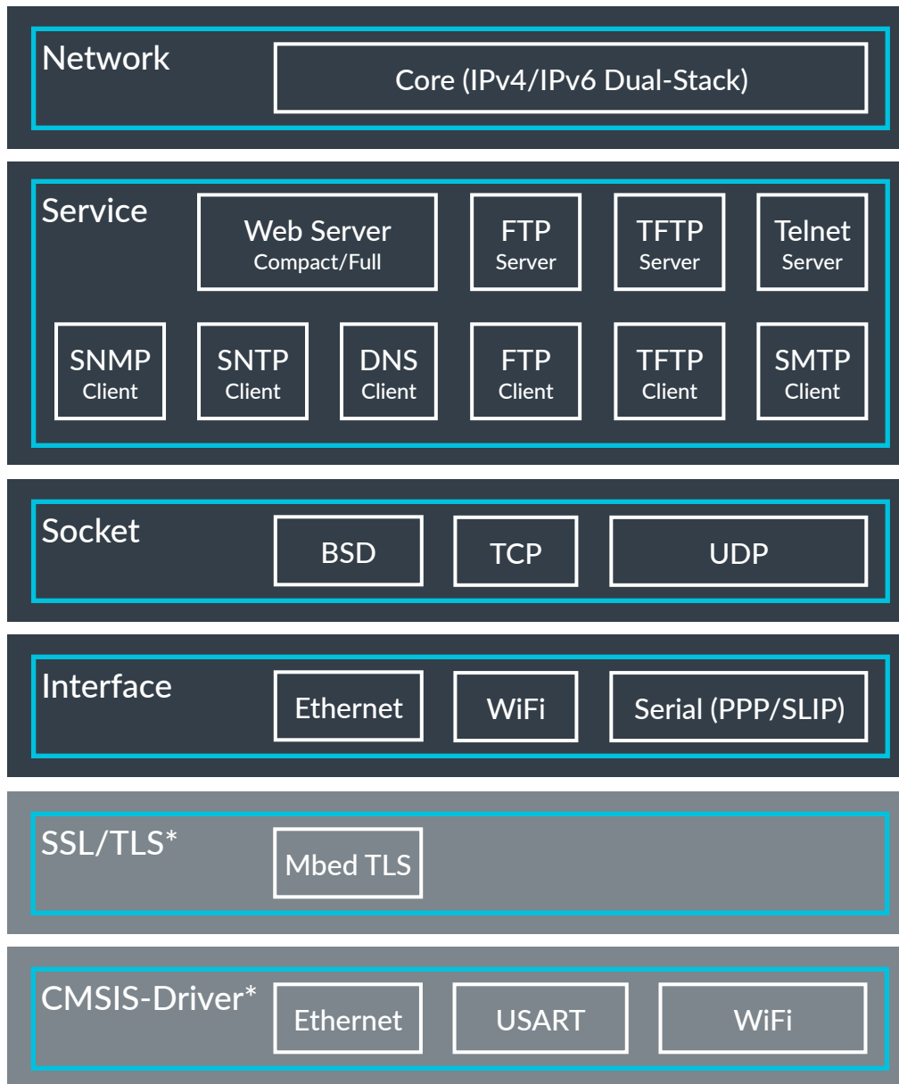
Figure 5-2: MDK-Middleware Network component overview diagram
