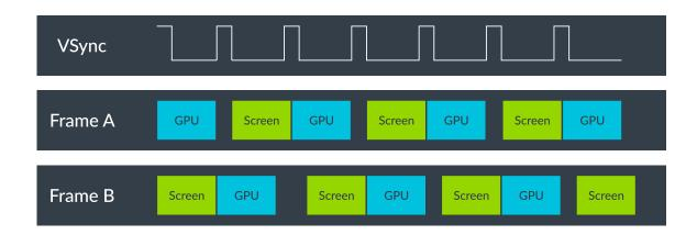
In a system using two buffers for a framebuffer – double-buffering – it is possible to have content which is not hitting 60 FPS but that is still limited by the vsync rate. This occurs because the GPU cannot modify a framebuffer which is still being scanned out to the display, and the GPU runs out of buffers to render in to.
