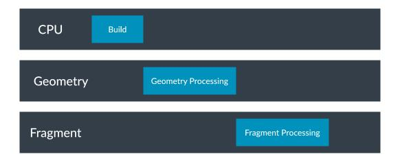
The processing time of each of the three component workloads of a render pass is not usually identical. A well scheduled workload which is processing limited will see the most heavily loaded pipeline stage running all of the time, and the other two going idle periodically waiting for the slowest stage to catch up. The swim lane diagram below shows the typical pipelining for two frames of content which is bottlenecked by fragment processing performance.
