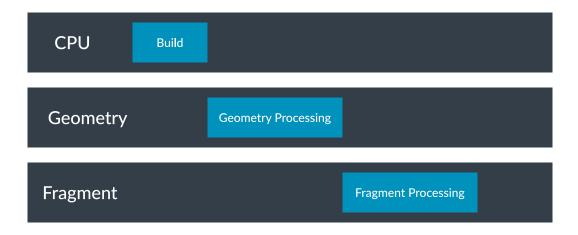
Note that this diagram shows each phase starting immediately after the previous one finishes, but in reality the three processing queues are decoupled. If a queue is busy processing an earlier render pass then there may be a delay in starting its workload.
