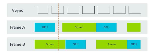
In this situation the user-visible frame rate will snap to an integer division of the vsync rate – i.e. 30 FPS, 20 FPS, 15 FPS, etc. – despite having a GPU which could render the application faster. If you see this issue it is recommended that you disable vsync locking while doing performing optimization because it will mask improvements and makes measuring progress difficult.
