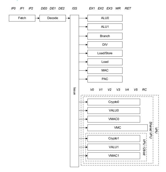
Figure 1 Cortex-A520 Core pipeline
