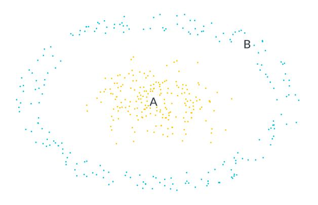
Cluster A and B cannot be separated by a plane. To solve this issue, SVM algorithms introduce nonlinear transformations.
