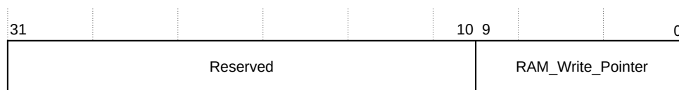
Figure 4-77: RWP register bit assignments
