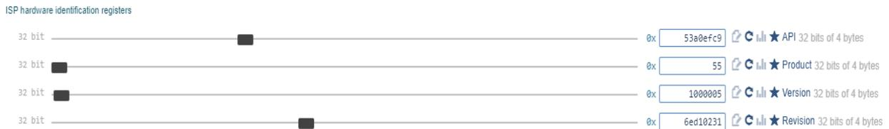
If the value read from ACT client does not match with the value defined in the register map document, you must check whether the porting implementation of the register read API is correct.
