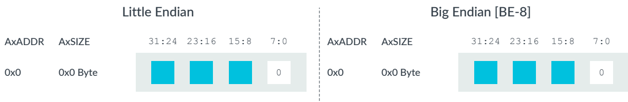
Figure 7-14: For a single byte, there is no difference between little-endian and big-endian mode
