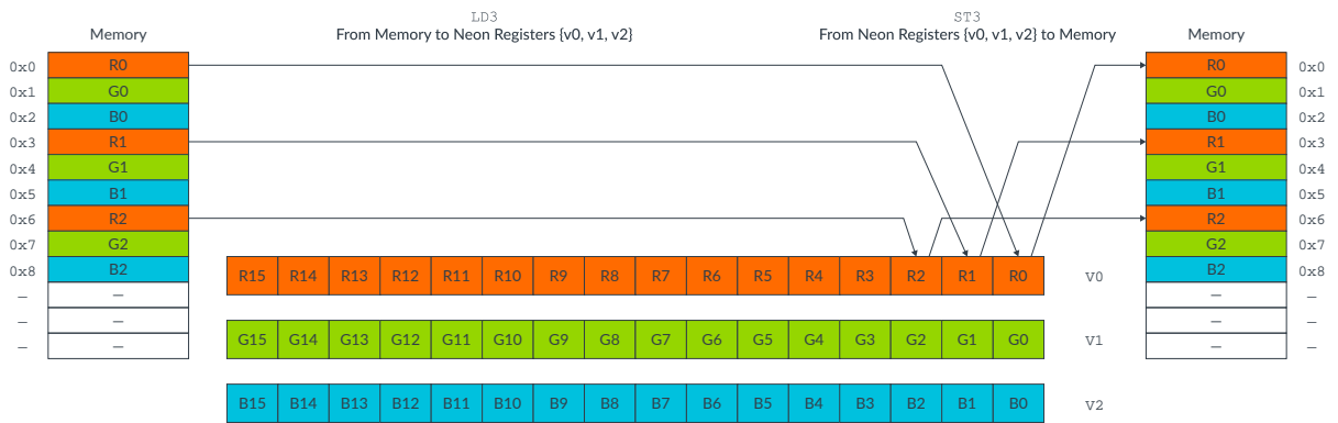
Figure 3-1: Interleaving store with ST3
