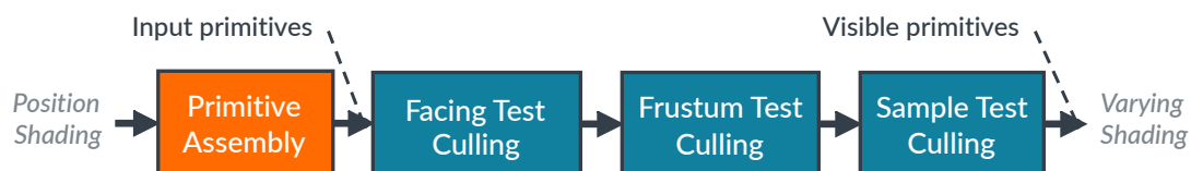
Figure 4-1: Valhall GPU culling pipeline
