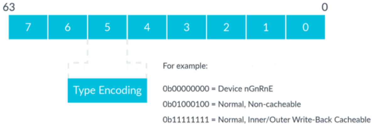
Figure 7-1: A diagram showing memory attribute indirection register.
