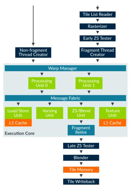
The Valhall programmable Execution Core (EC) consists of one or more Processing Engines (PEs). The Mali-G57 and Mali-G77 have two PEs, and several shared data processing units, all of which are linked by a messaging fabric.
