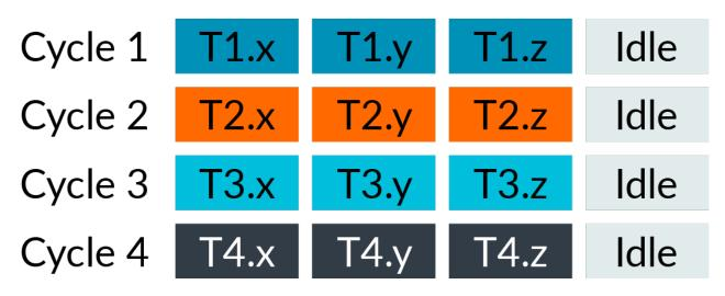
By contrast, in this example the pipeline in a 4-wide warp unit, executes one lane per thread for four threads per clock:
