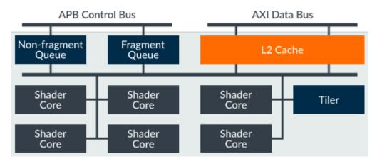
To improve performance, and to reduce memory bandwidth wastage that is caused by repeated data fetches, the shader cores in the system all share access to a level 2 cache. The size of the L2 cache is configurable by our silicon partners, is typically in the range of 64-128KB for each shader core in the GPU. However, the size of the L2 cache depends on how much silicon area is available.
