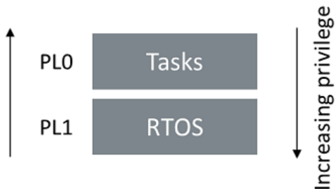
Figure 5-1: A diagram showing Armv7-R privilege
