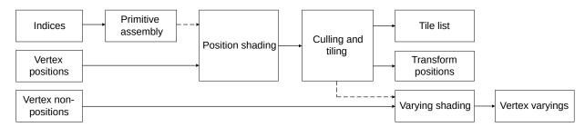
The position shader is executed for every index vertex, but the varying shader is only executed for vertices that are part of a visible primitive that survives culling. Mali Offline Compiler reports separate performance tables for each of these variants.
