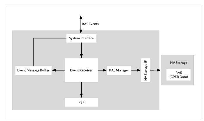
Figure 8: IPMI based RAS Event Receiver
