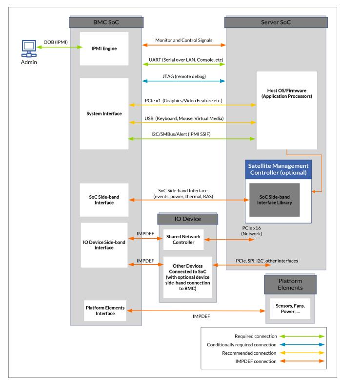
Figure 2: Server Management Interfaces (Level M1)
