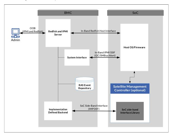
Figure 9: Redfish and IPMI based RAS Interfaces
