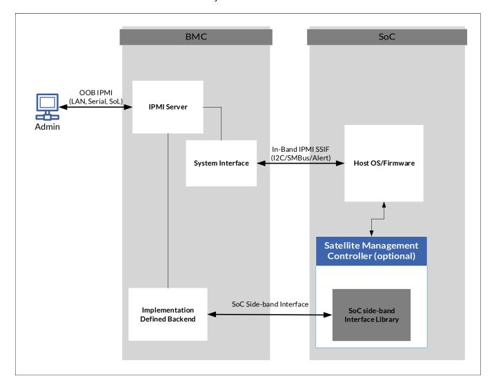
Figure 7: IPMI based RAS Interfaces
