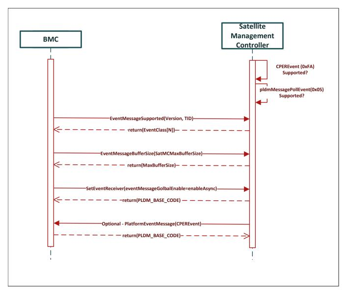
Figure 11: RAS side-band flow - boot initialization
