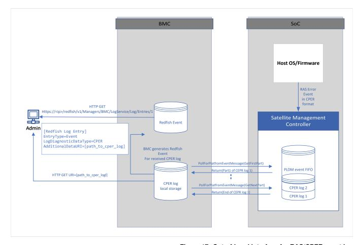
Figure 17: Out-of-band interface for RAS/CPER event log
