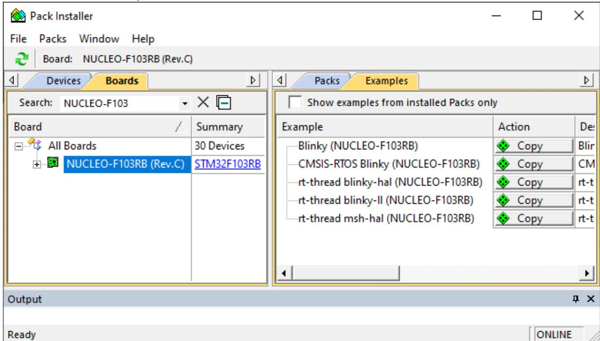
3. When pressing **Copy**, a dialog box will ask for the desired destination. The example will be directly installed into this folder. Folders that do not exist will be created automatically.
