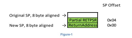
On a function return from Non-secure to Secure when a qualifying instruction, for example POP {pc}, loads PC with the FNC\_RETURN value, the stacked contents, partial RETPSR and ReturnAddress, are read back from the Secure stack frame. During this function return process, a set of *integrity checks* are performed.
