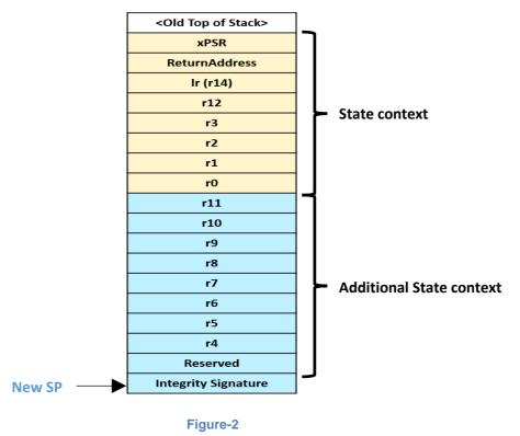
One important characteristic of the integrity signature is that it starts with 0xF but is not equal to FNC\_RETURN or EXC\_RETURN. This means that, in accordance with the Armv8-M architecture, any attempt to set the PC to this value will result in a MemManage fault. This is because addresses starting with 0xF are non-executable.
