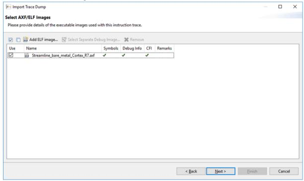
Streamline uses these files to decode the trace.
