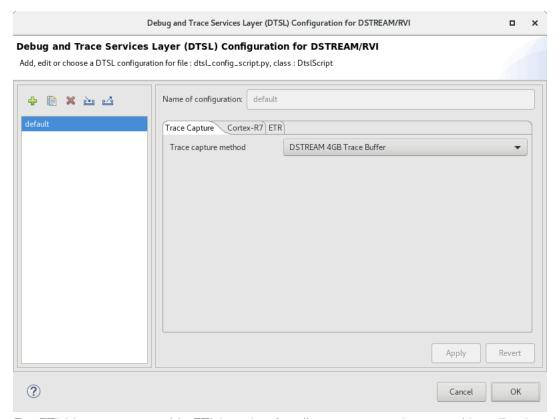
For ETM4, you must enable ETM tracing for all cores you are interested in collecting data from. On this tab, you can also enable data address tracing. If the **Enable ETM Timestamps** option is available, select it.
