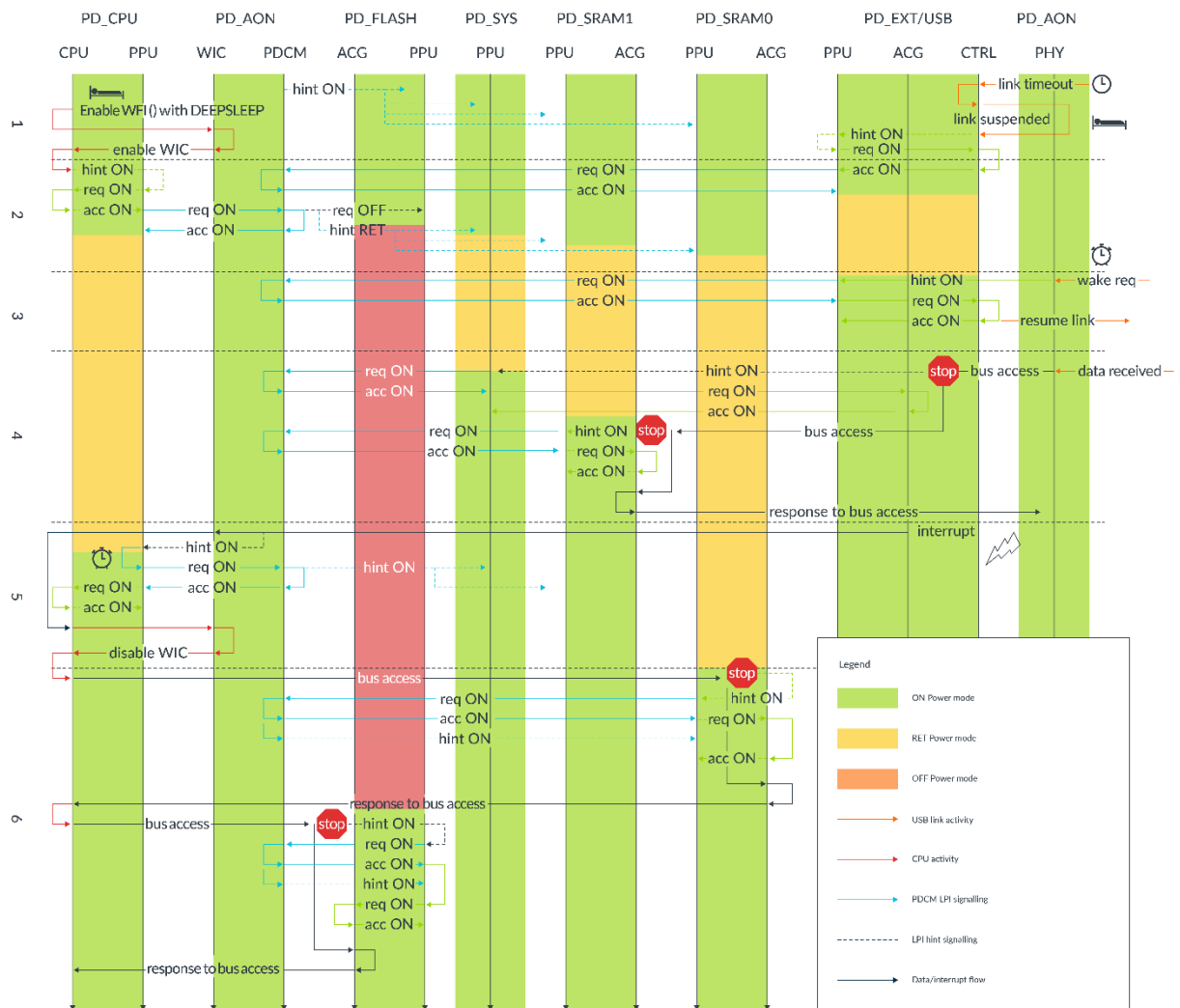
Figure 13: Software and hardware event flow
