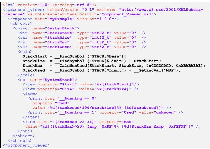
Add the SystemStack.svcd file to the debug session via Project – Options for Target – Debug – Manage Component Viewer Description Files. In a running debug session, open this view via View – Watch Windows – SystemStack:
