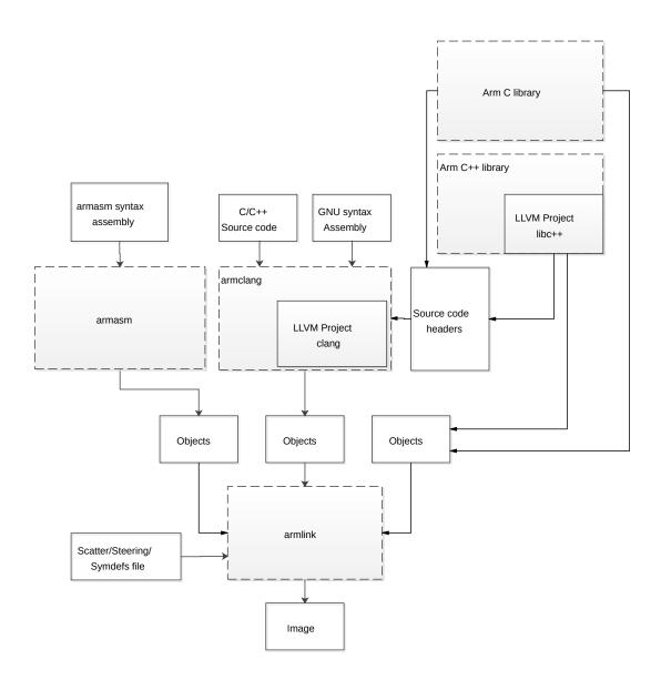
The dashed boxes are toolchain components, and any interaction between these components is an integration boundary. Community features that span an integration boundary might have significant limitations in functionality. The exception to this is if the interaction is codified in one of the standards supported by Arm Compiler for Embedded 6. See Application Binary Interface (ABI). Community features that do not span integration boundaries are more likely to work as expected.
