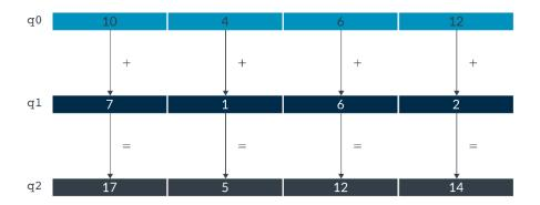
Being able to specify parallel operations in a single instruction like this allows the processor to do the calculations simultaneously, which increases performance and throughput. The preceding diagram shows 128-bit registers, with each register holding four 32-bit values. Operations on data elements with different data sizes are possible for Helium registers. We explain this in more detail in **Helium registers**.
