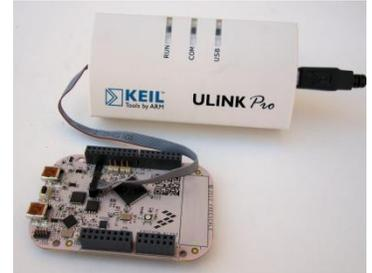
You can use OpenSDA on the Kinetis boards. For Serial Wire Viewer (SWV), a ULINK2, ULINK-ME or a J-Link is needed. For ETM support, a ULINKpro is needed. OS-JTAG or OpenSDA do not support SWV or ETM. KL25 does not have SWV.
