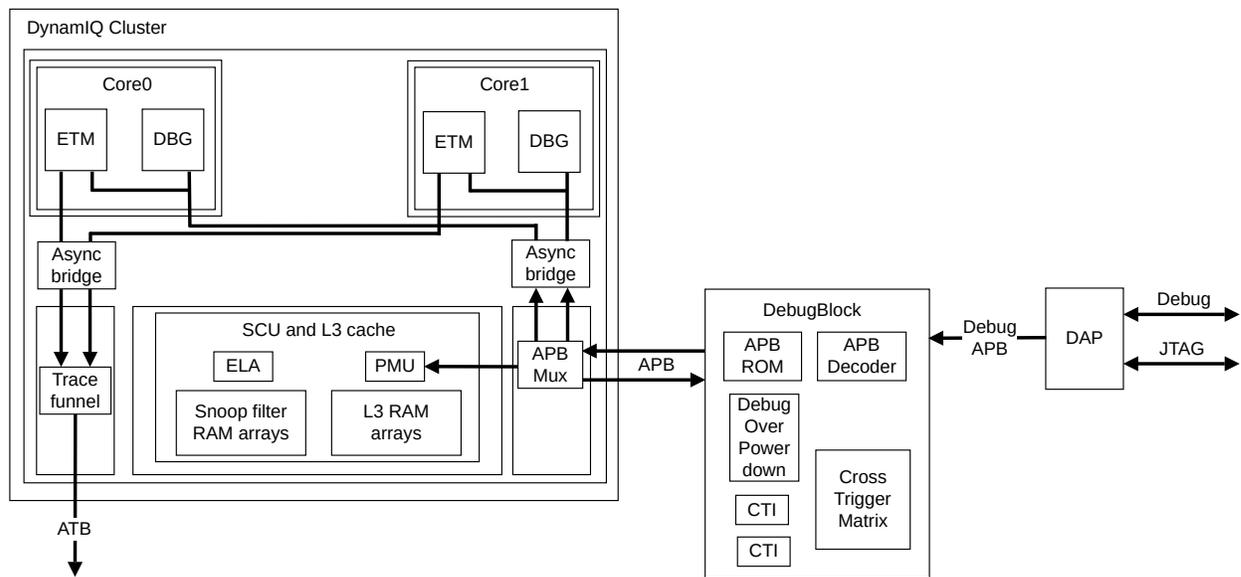
The primary debug APB interface on the DebugBlock controls the debug components. The APB decoder decodes the requests on this bus before they are sent to the appropriate component in the DebugBlock or in the DynamIQ™ cluster. The per-core CTIs are connected to a CTM.
