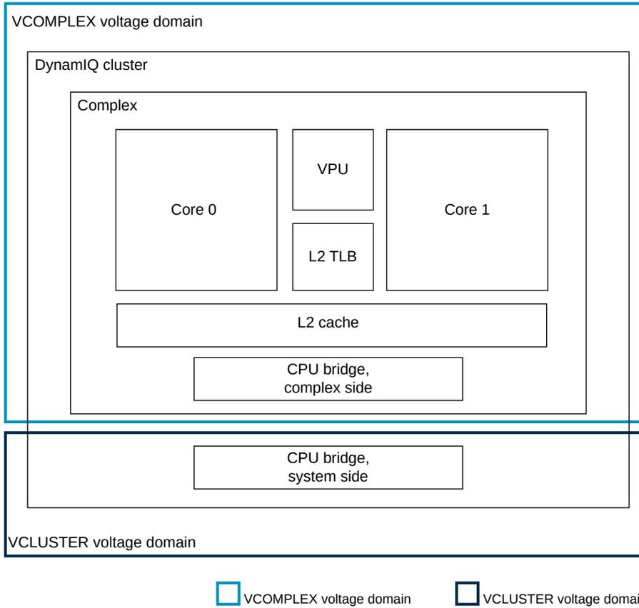
The following figure shows the power domains for an example Cortex®-A510 configuration with a dual-core complex:
