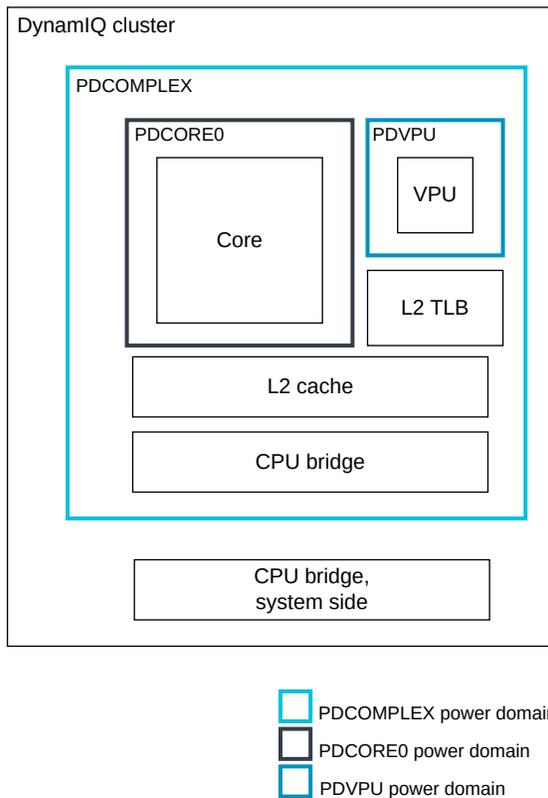
For a single-core complex, the voltage and power domains are similar to those for a dual-core complex. Within the PDCOMPLEX power domain, the single core is in PDCORE0, a gated power domain that can support retention. The core has its own dedicated logic, including a VPU within its own PDVPU power domain. The L2 TLB, the L2 cache, and the CPU bridge, complex side, is in the PDCOMPLEX power domain.
