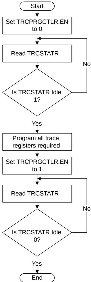
The following figure shows the flow for programming ETM registers using the System register interface:
