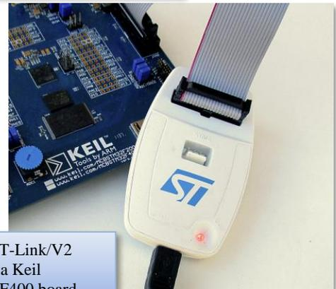
Standalone ST-Link/V2 connected to a Keil MCBSTM32F400 board.
