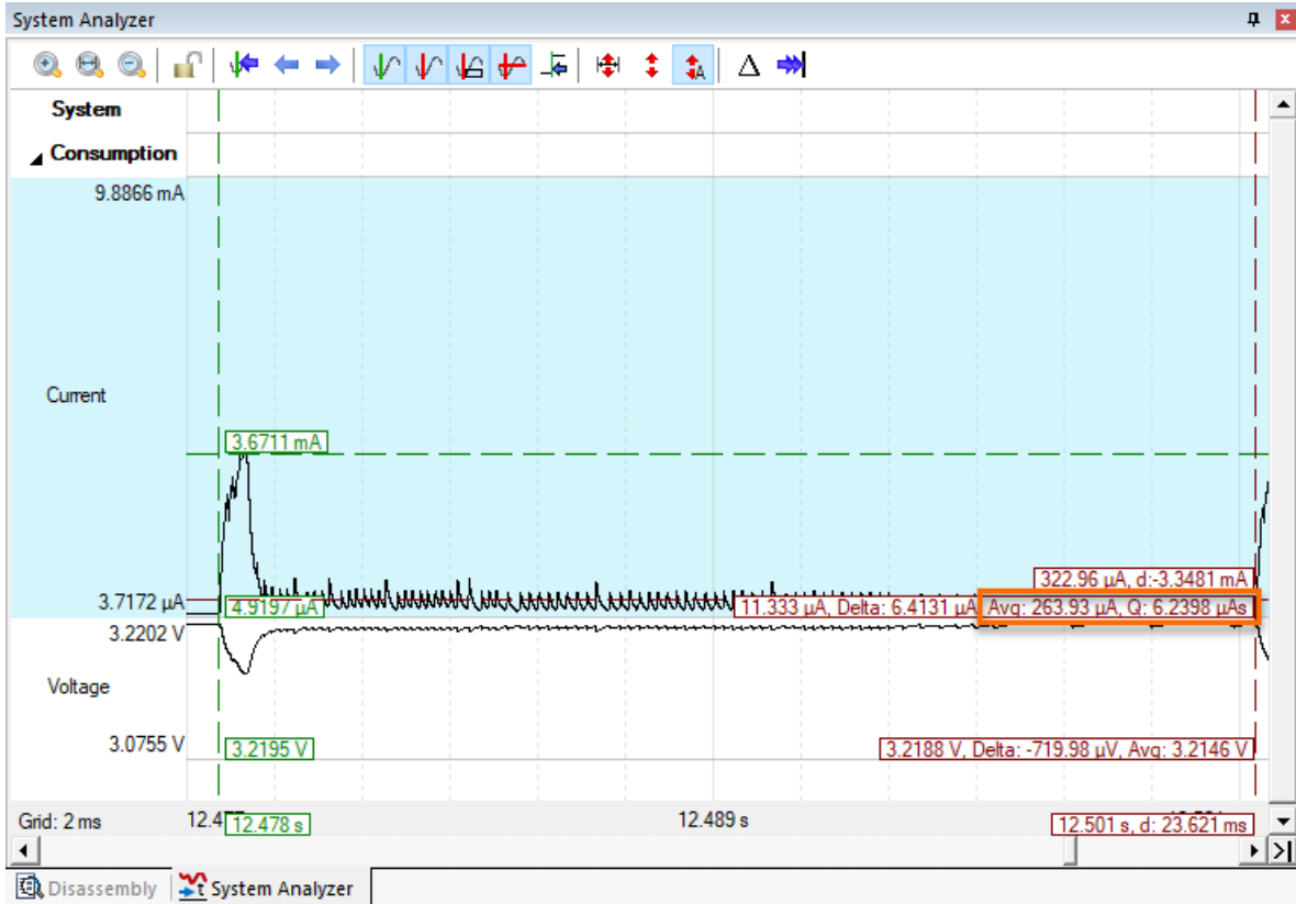
Figure 9 Power measurement profile for triggering sensors after software redesign
