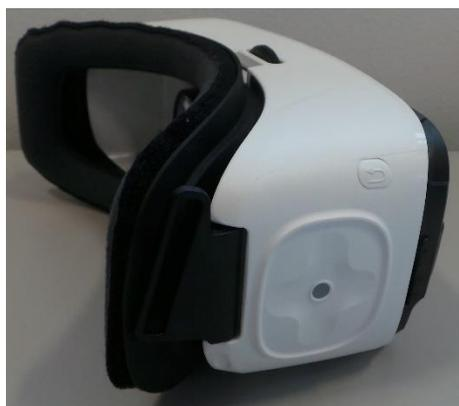
Figure 4. A Samsung Gear VR headset showing the touchpad
