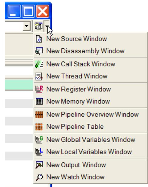
Figure 2-17 Icons for selecting a new debug view
