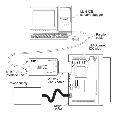
Figure 1-2 A typical debugging set-up
