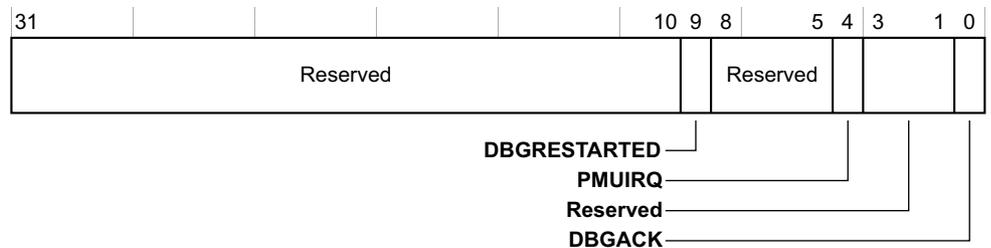
Figure 10-18 DBGITMISCOUT bit assignments
