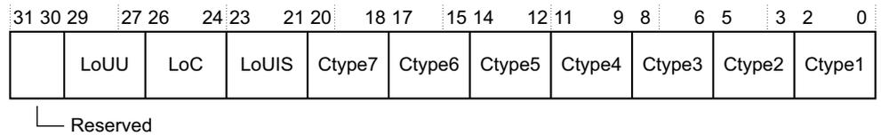
Figure 4-19 CLIDR bit assignments
