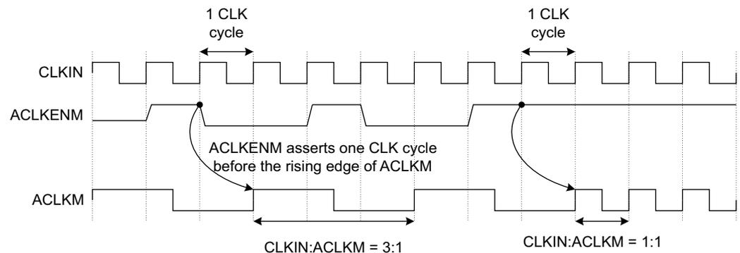
**Figure 2-2 ACLKENM with CLKIN:ACLKM ratio changing from 3:1 to 1:1**
