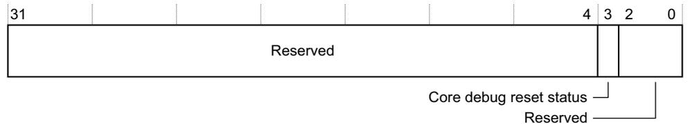
**Figure 10-5 DBGEACR bit assignments**
