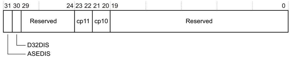
Figure 4-28 CPACR bit assignments
