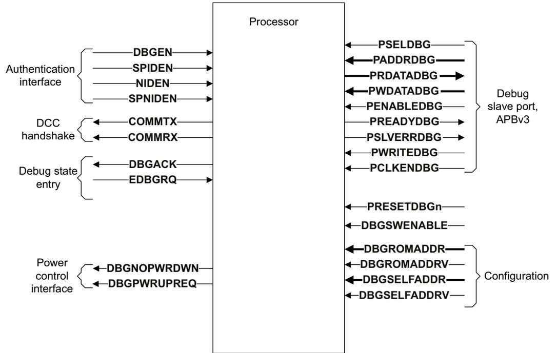
Figure 10-25 External debug interface, including APBv3 slave port
