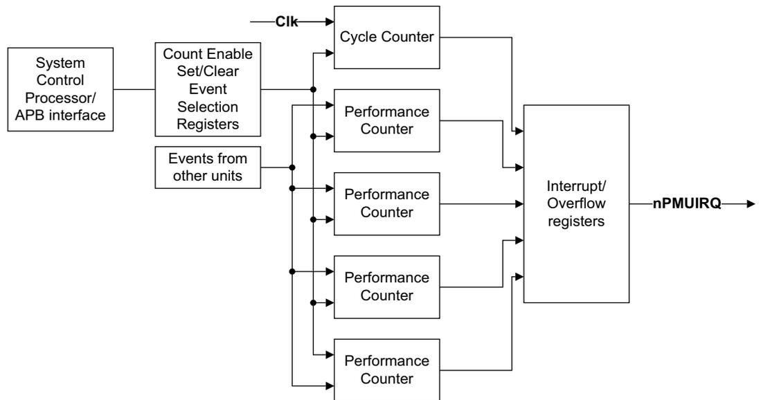
Figure 11-1 PMU block diagram
