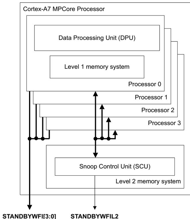
**Figure 2-6** STANDBYWFI[3:0] and STANDBYWFIL2 signals
