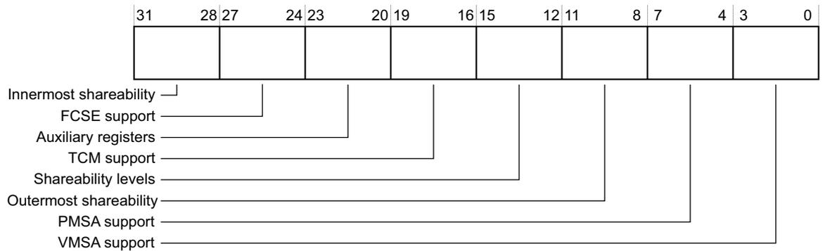
Figure 4-9 ID\_MMFR0 bit assignments
