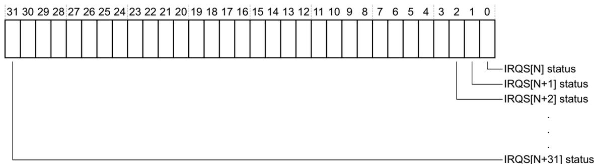
**Figure 8-4** GICD\_SPISRn bit assignments
