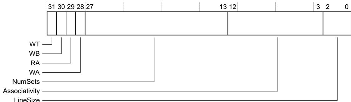
Figure 4-18 CCSIDR bit assignments
