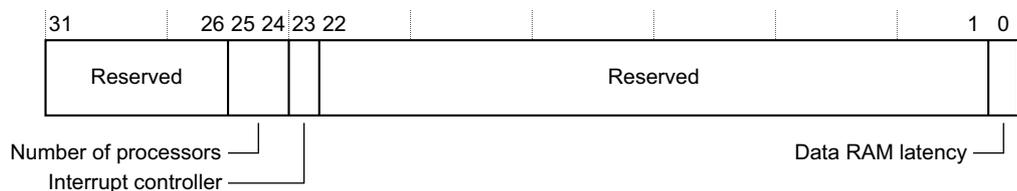
**Figure 4-39 L2CTLR bit assignments**
