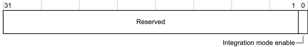
**Figure 10-20 DBGITCTRL bit assignments**
