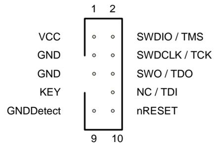
The Cortex Debug Connector supports JTAG debug, Serial Wire debug and Serial Wire Viewer (via SWO connection when Serial Wire debug mode is used) operations.
