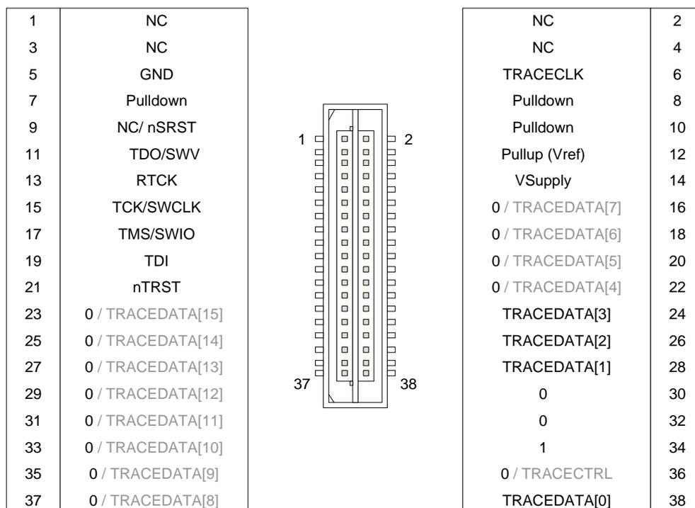
The Mictor connector is still the recommended trace connector for other ARM processors including ARM7, ARM9, Cortex-R and Cortex-A processors, and other applications that require wider trace widths (e.g multiple processors).
