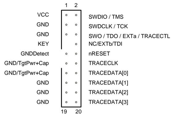
The Cortex Debug+ETM Connector supports JTAG debug, Serial-Wire debug, Serial Wire Viewer (via SWO connection when Serial Wire debug mode is used) and instruction trace operations.
