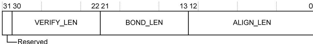
**Figure 15 : Link Layer Initialization Register bit assignments**
