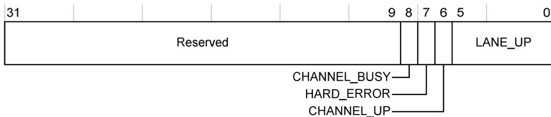
**Figure 11 : STP Status Register bit assignments**
