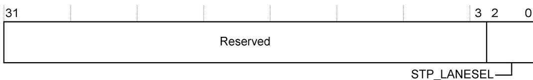
**Figure 13 : STP Lanes Select Register bit assignment**
