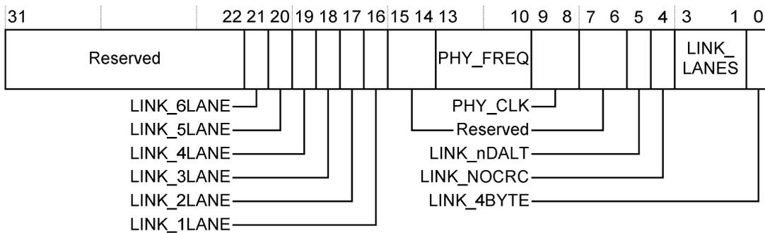
Figure 16 : LINK and PHY Capability Register bit assignments
