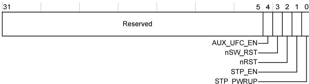
**Figure 12 : STP Control Register bit assignments**
