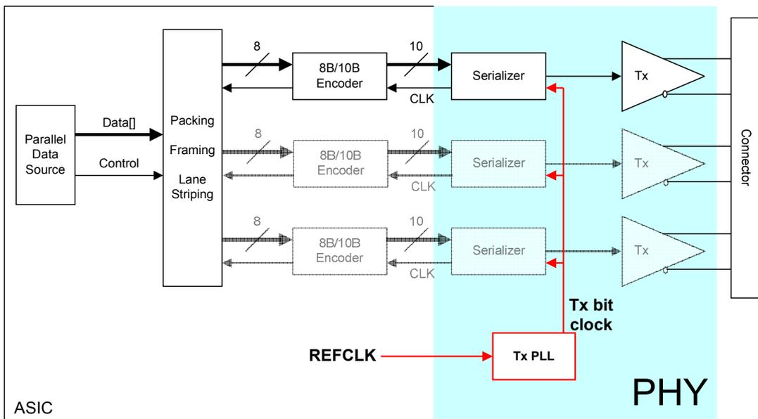
Figure 4 : Example configuration A – internal reference clock
