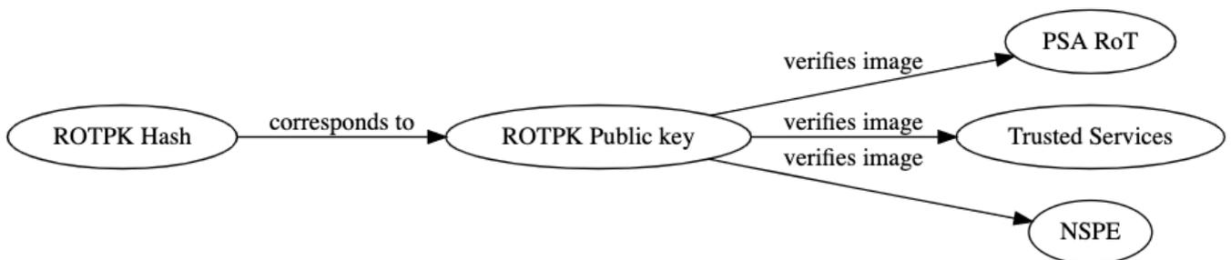
Figure 4: Single provider with a single signing key
