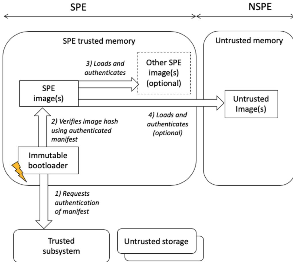
Figure 9: Example boot using a passive security subsystem
