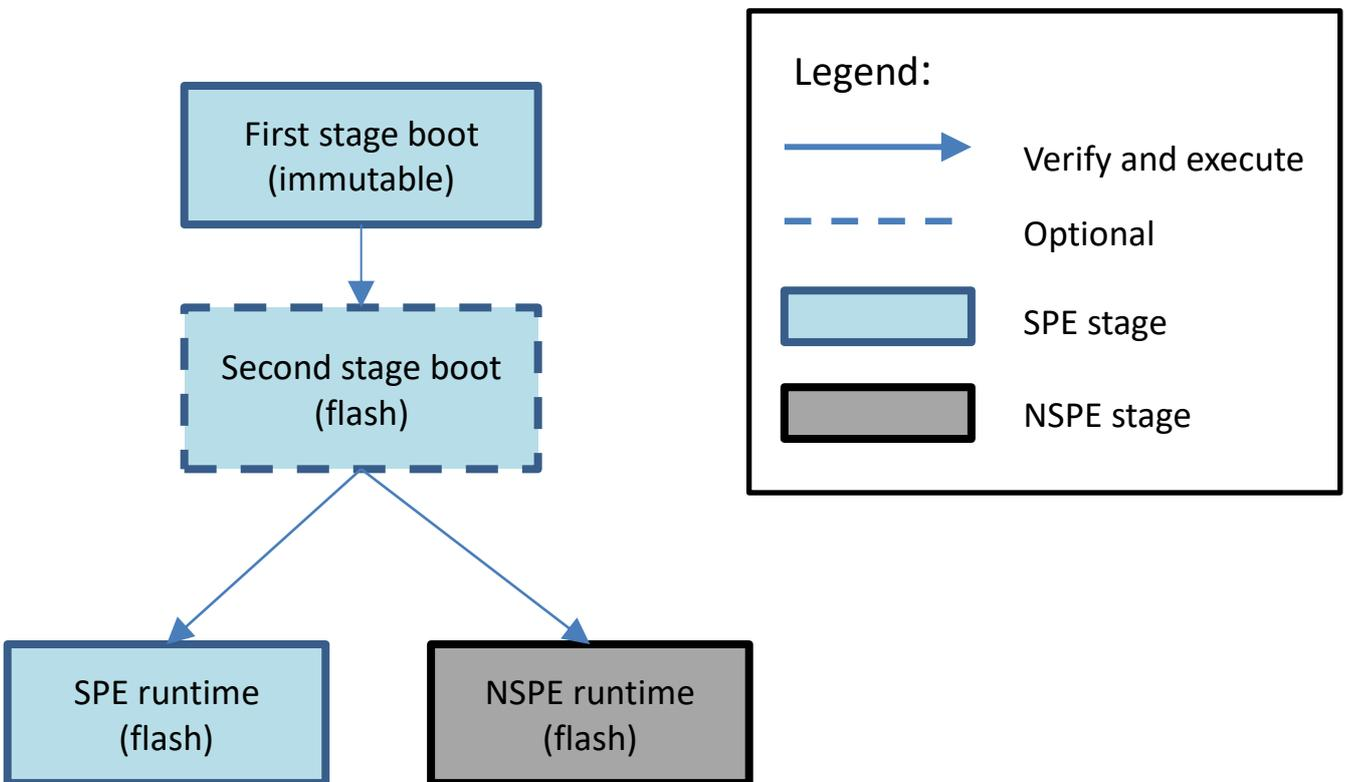
Figure 3: Generic boot process with multiple stages
