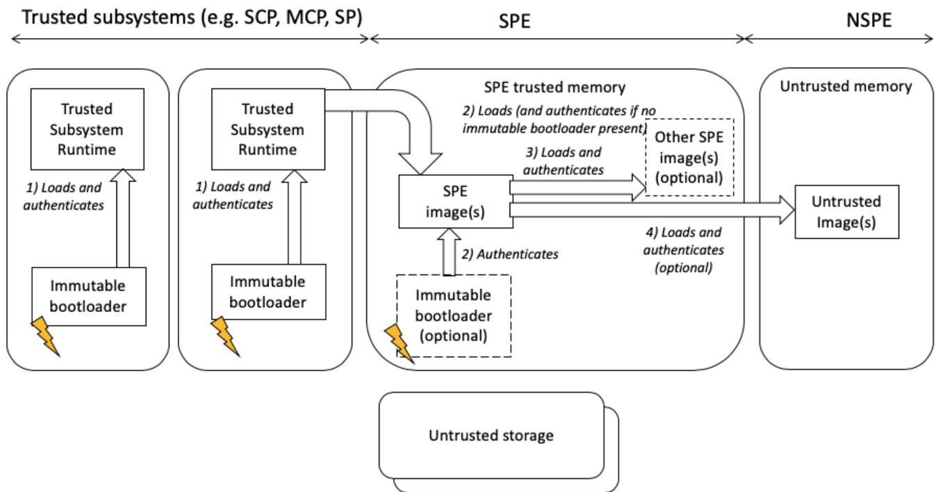
Figure 10: Example boot using a security subsystem that directly loads and verifies images in the SPE
