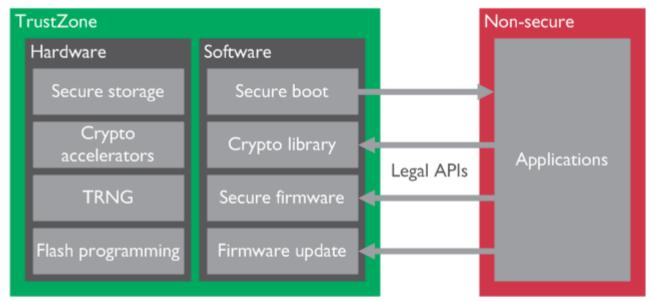
Figure 2-2 Security features in a microcontroller for IoT applications
