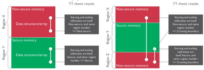
Figure 1-10 TT instruction allows software to determine if a data object is placed entirely in a Nonsecure region
