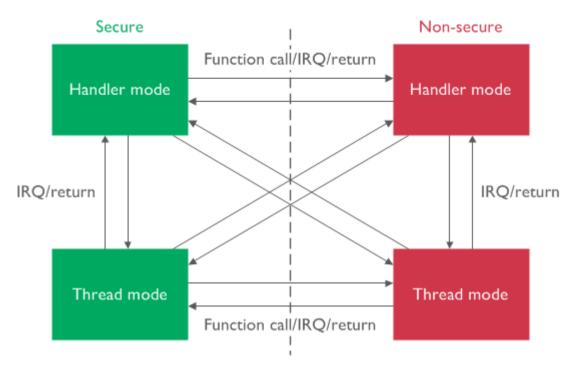
Figure 1-9 Forms of transition between Secure and Non-secure worlds
