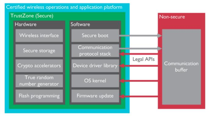
Figure 2-3 Protecting the operation of a wireless communications interface
