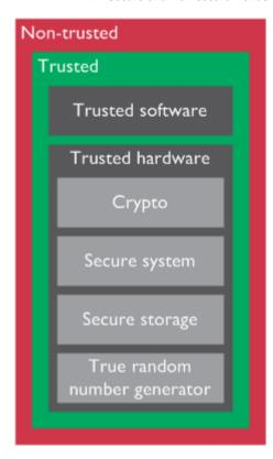
Figure 1-2 Secure and Non-secure worlds
