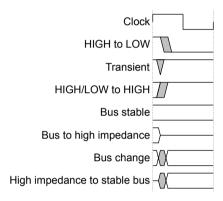
Figure 1 Key to timing diagram conventions
