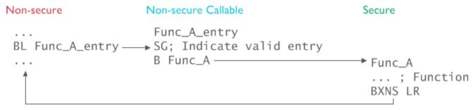
Figure 1-7 Software flow when a Non-secure program calls a function in the Secure world
