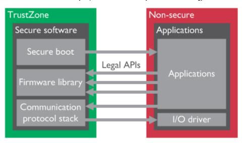
Figure 2-1 A simple use case of TrustZone technology for ARMv8-M showing firmware protection
