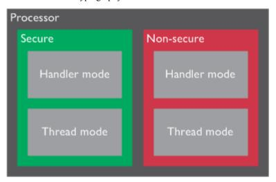
Figure 1-1 TrustZone technology for ARMv8-M adds Secure and Non-secure states to processor operation
