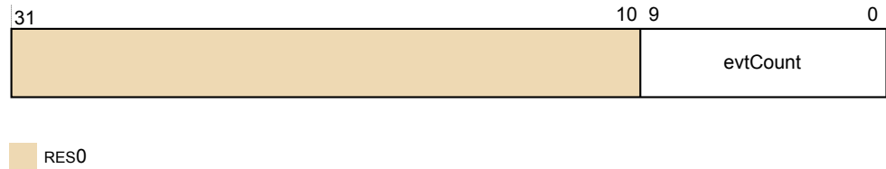
Figure D8-6 AMEVTYPERN_EL0 bit assignments
