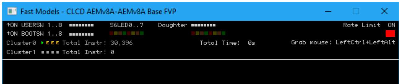
Figure 2-2 Core run state icons for a dual-cluster, quad-core model
