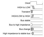
Figure 1 Key to timing diagram conventions
