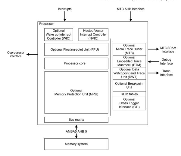
Figure 1-1 Cortex-M33 processor implementation without the Security Extension
