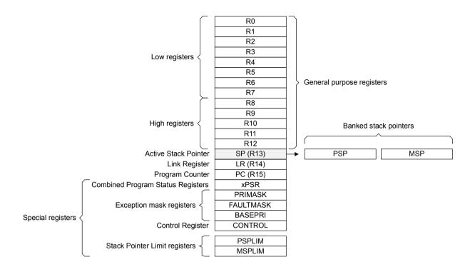
Figure 2-1 Core registers without the Security Extension
