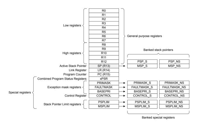
Figure 2-2 Core registers with the Security Extension
