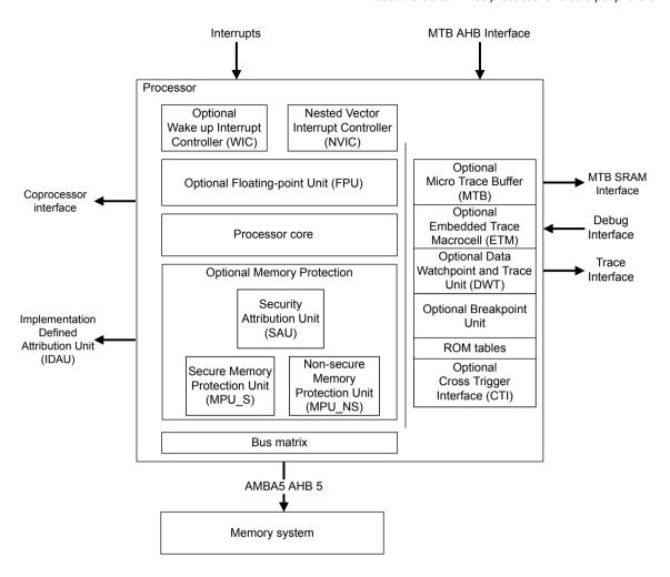
Figure 1-2 Cortex-M33 processor implementation with the Security Extension
