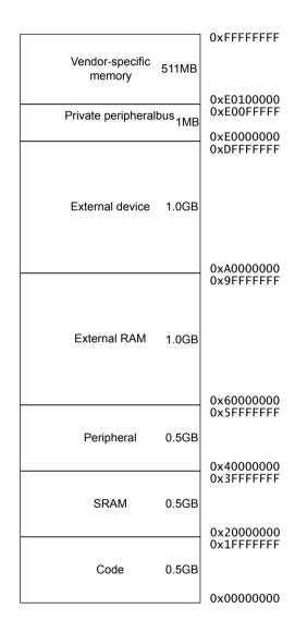
Figure 2-3 Cortex-M33 processor memory map
