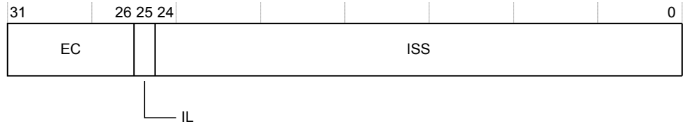
Figure B2-46 ESR_EL1 bit assignments
