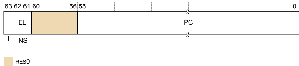
Figure D7-1 PMPCSSR bit assignments
