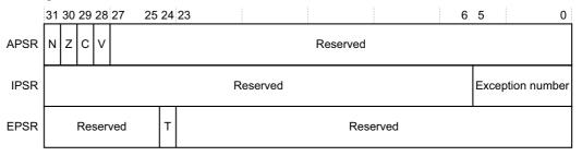
b. Bit[24] is the T-bit and is loaded from bit[0] of the reset vector.
