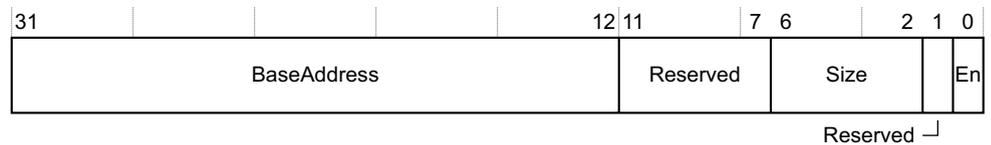
**Figure 4-58 Peripheral Interface Region Register bit assignments**
