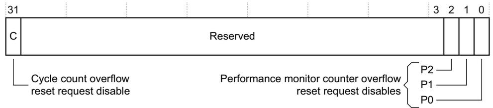
**Figure 4-50 nVAL Reset Enable Clear Register bit assignments**
