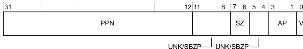
Figure 4-25 TLB PA Register bit assignments
