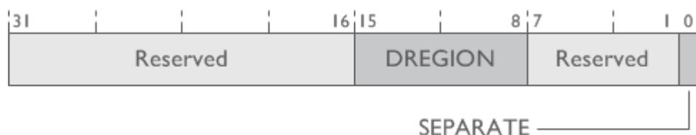
Figure 4-1 MPU\_TYPE bit assignments
