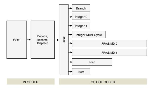
The execution pipelines support different types of operations, as shown below.
